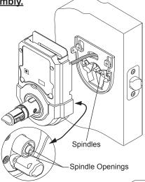
**b.** Once flush on door, insert and tighten small screws to secure assembly onto the mounting plate.
